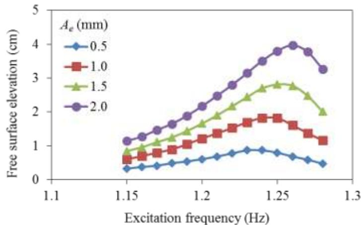
Fig.3: Free surface elevation as a function of frequency at right wall of tank without baffles for different excitation amplitudes when  $h_0 = 70$  mm (with the oil).
