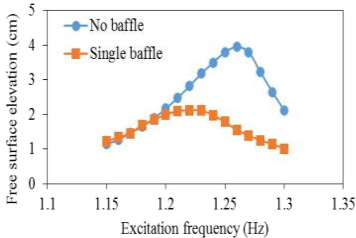
Fig. 6: Free surface elevation as a function of excitation frequency at right wall with/without baffles when  $h_0 = 70$  mm and  $A_e = 2$  mm (with the oil).
