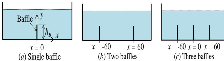
Fig.5: Baffle arrangements (Units: mm).
