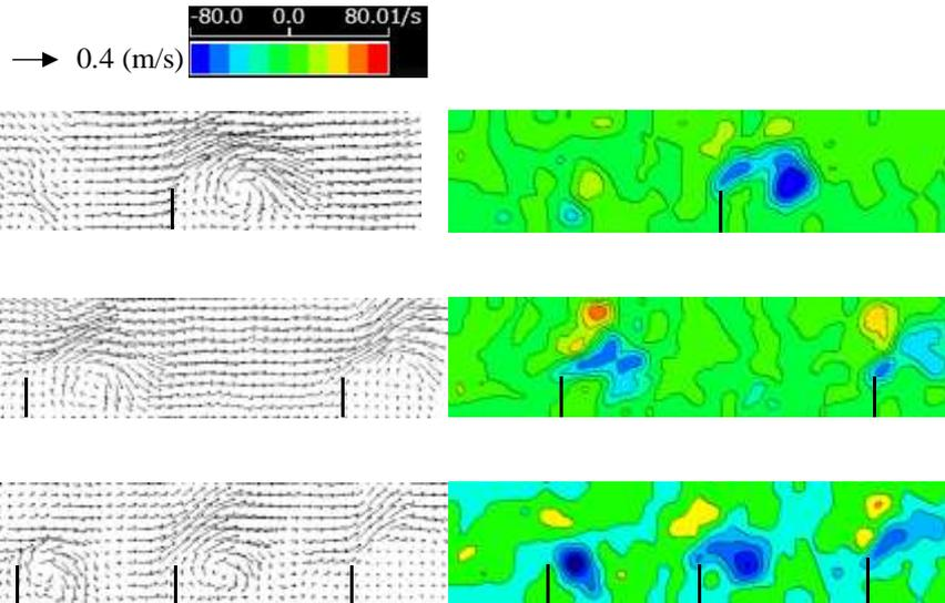
Fig. 10: Velocity vectors (left) and vorticity contours (right) obtained by PIV in the vicinity of baffles at  $T/4$  when  $h_0 = 60$  mm,  $\omega_e = 7.5$  rad/s, and  $A_e = 2$  mm (with water).
