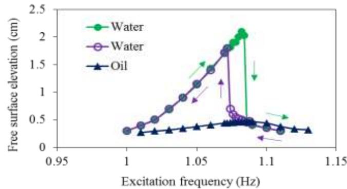
Fig.2: Free surface elevation as a function of excitation frequency at right wall of tank without baffle when  $h_0 = 50$  mm and  $A_e = 0.5$  mm in the cases with water and the oil. The solid circles indicate an increase in the frequency while the open circles indicate a decrease in the frequency in the case of water. The triangles indicate an increase and a decrease in the frequency for the oil.
