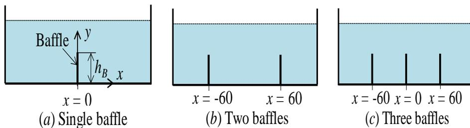
Fig.5: Baffle arrangements (Units: mm).
