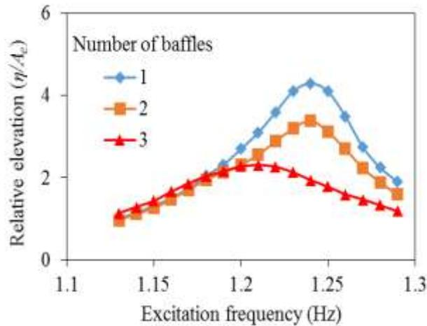
**Fig.8:** Relative free surface elevation as a function of excitation amplitude with different numbers of baffles when  $h_0 = 50$  mm and  $A_e = 2$  mm (for water).
