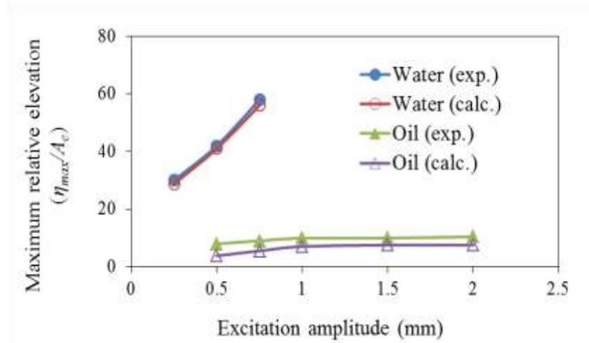
Fig.4: Maximum relative free surface elevation as a function of excitation amplitude at right wall of tank without baffle when  $h_0 = 70$  mm (for water and the oil).
