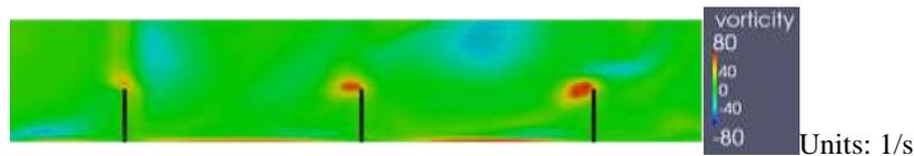
Fig. 11: Vorticity contour obtained numerically by OpenFoam in the vicinity of the baffles at  $T/4$  when  $h_0 = 60$  mm,  $\omega_e = 7.5$  rad/s, and  $A_e = 2$  mm.
