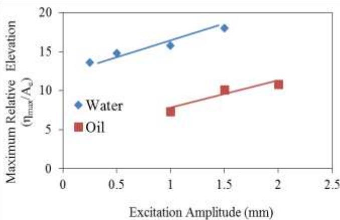
**Fig.9:** Relative maximum free surface elevation as a function of excitation amplitude at right wall of tank with single baffle when  $h_0 = 70$  mm (both water and the oil).
