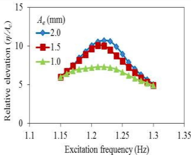
Fig.7: Relative free surface elevation as a function of excitation frequency at right wall of tank with single baffle under different excitation amplitudes when  $h_0 = 70$  mm (with the oil).
